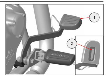
Push fit the GMA brake pedal rubber (1).
