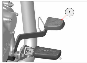
Remove the gear shifter rubber (1).
