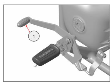
Push fit the GMA gear shifter rubber (1).
