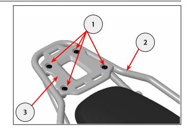
**2** Place the new top plate (1) onto the rear rack. Fit the four fixings from the kit (2). Tighten to **13Nm**.
