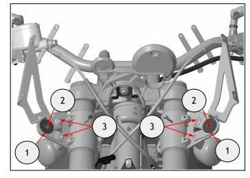
**6** Fix the headlamp assembly (1) onto the mounts (2) using the M8 x 25mm fixings (3) removed in step 2.
