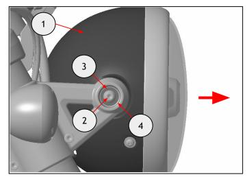
**3** Loosen the headlamp brackets (1) front fixings (2). Rotate the brackets outward.
