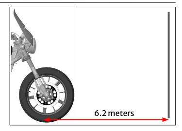
Ensure the motorcycle is perpendicular to the wall and upright.
