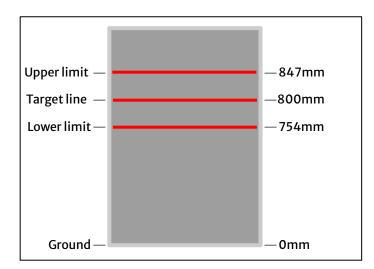
If the low beam criteria is not met, adjust the headlight angle using the adjuster bolt (1) and test again.
