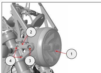
**7** Assemble the Touring Screen (1) on the brackets (2) using the M5 x 16mm fixings (3) from the kit. Tighten the fixings (3) to **5Nm**.
