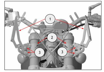
**5** Fit the two large rubber grommets (1) from the kit through the headlamp and screen brackets, then fit the top hats (2) removed in step 2 into the rubber grommets (1).
