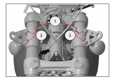
4 Loosely fit the two brackets (1) on the headlight mounts (2) using the M5 x 10mm fixings (3) from the kit.
