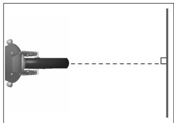
Turn the low beam on, the top of the beam must be between the two limit lines and as close to the target as possible.
