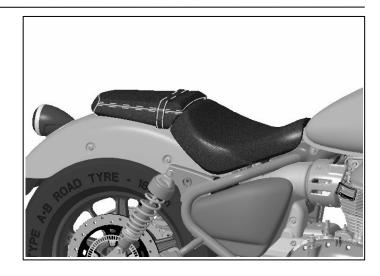
**2** Remove the pillion seat brackets (1) by removing the fixings (2).
