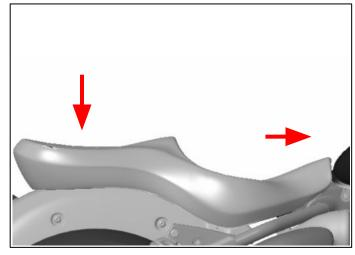
**5** Align the seat (1) with the rear bracket (2). Fit the M8 x 16mm fixing (3) removed in step 1. Tighten the fixing (3) to 18 Nm.
