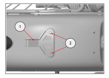
**4** Hook the front of the seat to the tank then push down on the seat to put it in place.
