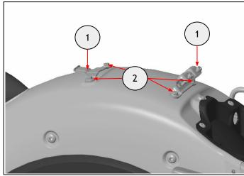
**3** Fit the seat bracket (1) onto the mudguard using the fixings (2) removed in step 2. Tighten the fixings (2) to **18Nm**.
