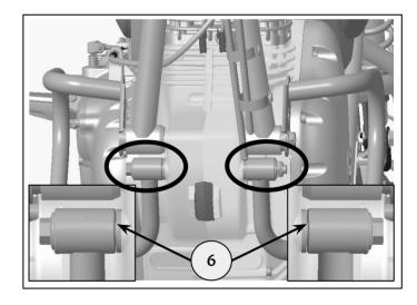
4 Position Exhaust pipe assembly to Engine head and silencer assembly as shown, Reuse the fixings (2),(3), and nut(4) retained in step 2. Connect the O2 sensor cable (1) to vehicle.
