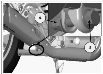
**2** Remove dust cap (1) on both sides to remove fixing (2), Washer and nut (3) from the vehicle cradle assembly as shown. Discard fixing, washer and nut.
