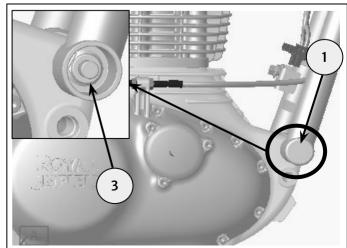
**3** Use Engine guard Left Hand (1), Engine guard right Hand (2) from the kit. position with vehicle cradle assembly. From the kit use M10 X 215mm fixing (3) and M10 nut (5) on the top.
