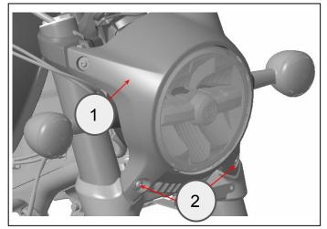
**9** Remove the headlamp housing fixings (1). Remove the housing from the upper rubber grommets (2). Rotate the housing forward. Move the throttle cables (3) under the upper fixing (2).
