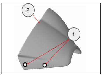
${f 2}$  Fit two rubber grommets (1) into the Flyscreen (2).
