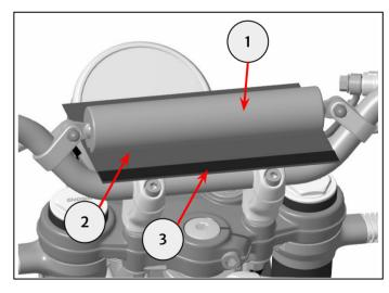
**4** Wrap the cover around the foam and overlap the hook and loop fastener.
