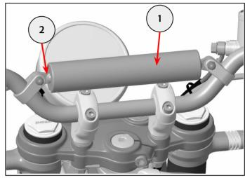
**3** With the foam (1) in place, place the cover (2) as shown with the hook fastener facing upwards (3).
