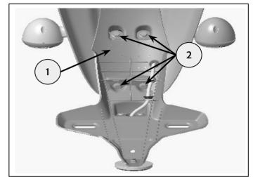
**25** Reassemble rear mudguard assembly to vehicle using the retained fixings(1), (2), and (3) and nut (4) retained from step 12. Tighten to **10Nm**.
