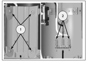
**11** Remove both left and right side existing indicators from mud flap by loosening the nuts (1), retain nuts for reuse.
