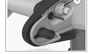
**7** Refit headlamp assembly with bracket, tighten to **10Nm** using fixings (1), nuts (2) and washers (3) retained in step 3 (hold the nut (2) from inside of the headlamp assembly). Do the process on both right and left hand side.
