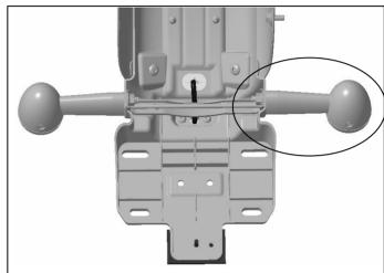
**18** Connect the three connectors (2) with vehicle harness (green to green and red to red). Fit the mudflap to the mudguard using the fixings and washers (1) retained from step 10 and tighten it to **10Nm**. (Use washer 2 Nos at top side only).
