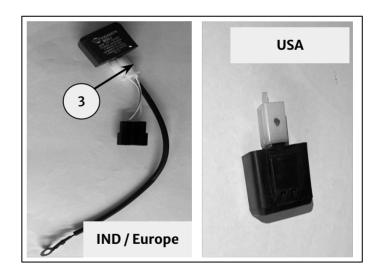
**28 IND and Europe:** Connect 2 pin connector from flasher unit with vehicle harness (1) as shown.
