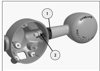
**20** Repeat step 19 on left side of the tail lamp housing using accessory indicator with red colour connector.
