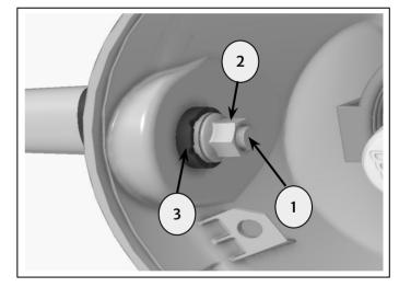
**8** Insert indicator connectors to vehicle connectors (red to red and green to green) inside the headlamp assembly. Refit the cover (1) inside the headlamp assembly, using fixings (2) retained in step 2.
