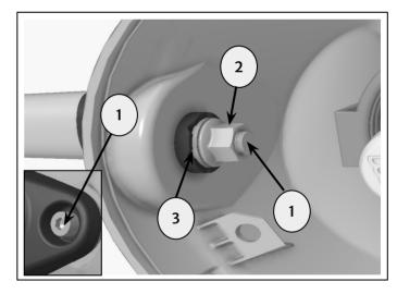
**4** Rotate right hand bracket (1) outwards, remove indicator from mounting bracket by loosening the nut (2). Repeat the step for left hand side. Retain the nuts for reuse.
