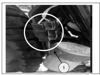
**29** Position Anti-rotation hole and align the mounting hole of flasher mounting bracket assembly (2) unit with Piece mudguard (1) as shown. Reuse fixing and washer(3) from step 26. Tighten to **6Nm**.
