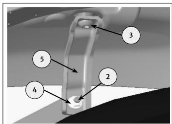
**13** Remove mud flap (1) from rear mudguard assembly by loosening the fixings (2) and disconnecting tail lamp assembly harness connectors (3), number plate harness (5) with rear body harness (4). Retain fixings (2) for reuse.
