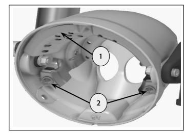
**9** Refit the headlamp (1) to headlamp assembly using fixings (2) retained in step 2, tighten to **5Nm**.
