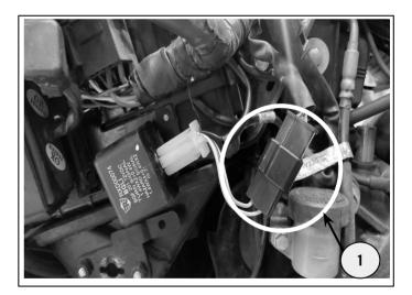
**35 IND and Europe:** Connect flasher's extension Negative terminal cable with battery as shown. Ensure proper cable routing as shown.
