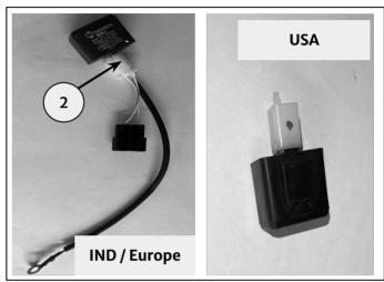
**34 IND and Europe:** Connect 2 pin connector from flasher unit with vehicle harness (1) as shown.
