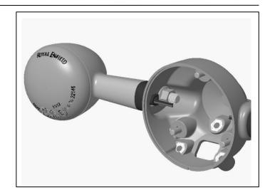
**21** Refit the tail lamp to tail lamp housing using retained fixings(1) from step 15. Tighten to **3Nm**.
