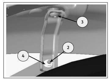
**26** Remove and retain fixing and washer set (3) to loosen flasher mounting bracket assembly unit (2). Remove fixings (4) and fixing (5) to loosen Piece mudguard (1), allow it to hang as it is.
