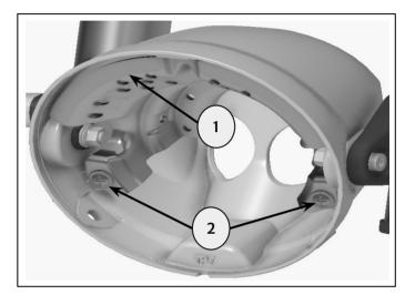
**3** Remove the fixing (1), nut (2) and washer (3) from right hand side of the headlamp mounting bracket, (hold the nut from inside the headlamp assembly). Retain the fixing, washer and nut for reuse. Repeat step for left hand side indicator.
