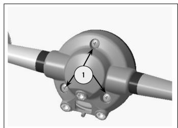
**22** Mount tail lamp housing(2) to mudguard using the retained fixing(3) from step 14,Route the connector through center hole available in the mudguard (1). Ensure anti-rotation feature on tail lamp assembly aligned with mudguard opening as shown. Tighten the fixing to **8Nm**.
