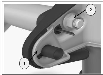
**5** Insert the M8 stud fixing (1) from the kit to the accessory indicator and tighten to **6Nm**. Insert an isolator (2) from the kit over the fixing as shown. Repeat step for the remaining indicators.
