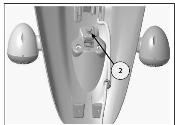
**15** Remove fixings(1) to open tail lamp housing, then remove existing indicators on both left and right hand side by loosening nut (2), retain for reuse.
