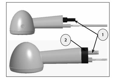
**6** Assemble indicator with red colour connector to the right hand side bracket, tighten to **6Nm** using the nut (1) retained in step 4. Use a 24mm spanner just to hold the indicator and isolator (Do not apply pressure on spanner). Repeat step for left hand side using indicator with green colour connector.
