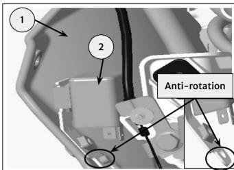
**30 IND and Europe:** Route flasher negative terminal cable (3) beneath seat unlock cable (3) and through over the battery as shown. Reuse fixing M6 x 16 (2) retained from step 26 to mount Piece mudguard (1) as shown. Tighten to 5 Nm.
