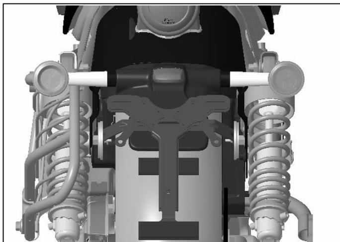
**35** To replace the flasher unit, remove the rider seat as described in the owner's manual.
