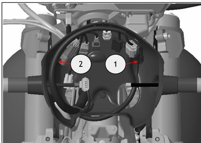
**32** Refit the cover (1) using the fixing (2) removed in step 26.
