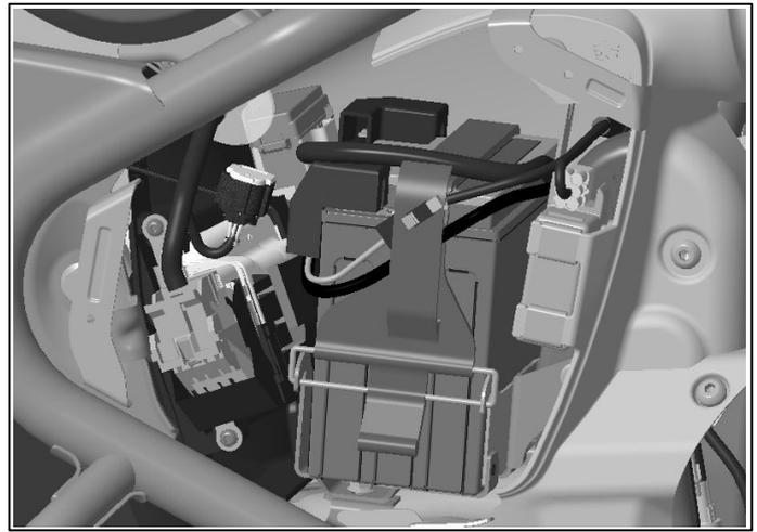
**2** Remove the headlamp assembly (1) by removing the fixings (2). Disconnect the headlamp connector. Retain both for reuse.
