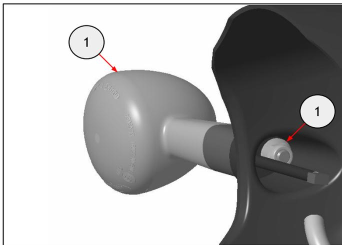
**29** Fit the studs (1) onto the indicators (2).
