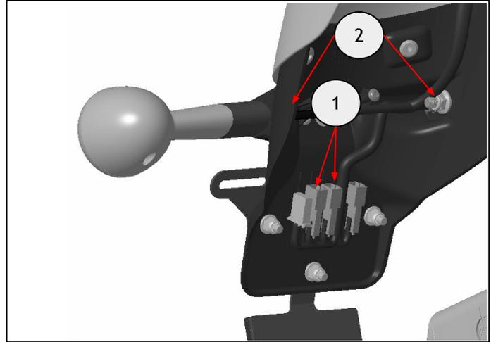
**16** Fit the studs (1) onto the indicators (2).
