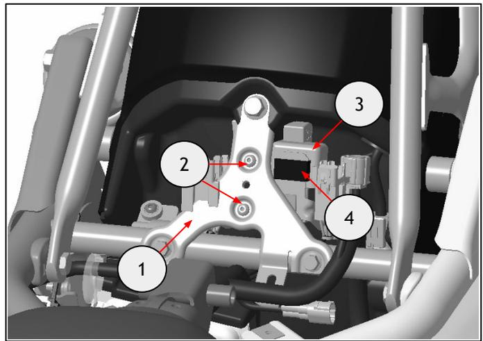
**37** Remove the extension wiring (1), which is not required for this model.
