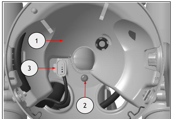
**13** Refit the headlamp assembly (1) using the fixings (2) removed in step 2.
