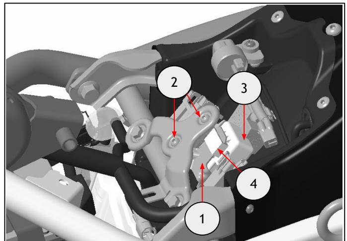
**21** Remove the extension wiring (1), which is not required for this model. Connect the flasher unit (2) into the factory connector then refit the rubber belt (3) to secure the new unit. Fix the flasher bracket (4) using the fixings (5) removed in step 20.
