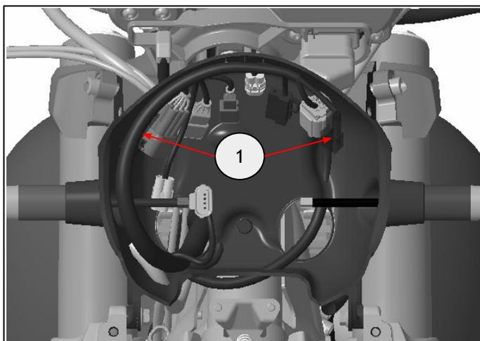
**28** Remove the factory indicator (1) by removing the nut (2).
