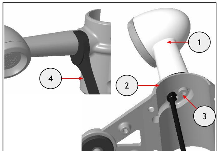
**9** Fit the indicator cable through the groove (1). Fit the headlamp mount (2) on the suspension fork using the M6 x 14 mm fixings (3) removed in step 5. Fix the headlamp using the M8 x 25 mm fixings (4) removed in step 5. Tighten the mount fixings (3) to **10Nm**. Tighten the headlamp fixing (4) to **10Nm**.
