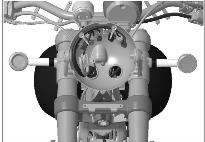
**11** Feed the indicator cables back through the holes in the headlamp bowl and reconnect the left indicator on the green connector (1) and the right indicator on the red connector (2).
