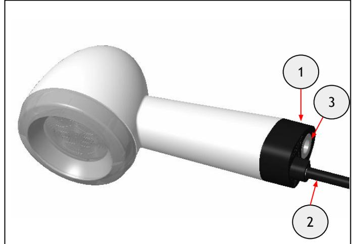
**8** Fit the indicator (1) onto the headlamp mount (2) using the fixing (3) from the kit. While maintaining the indicator in position using a 24mm spanner (4), tighten the fixing to 5Nm.
