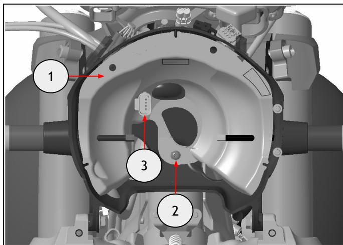
**33** Refit the casquette and headlamp assembly (1) using the fixings (2) removed in step 25.
