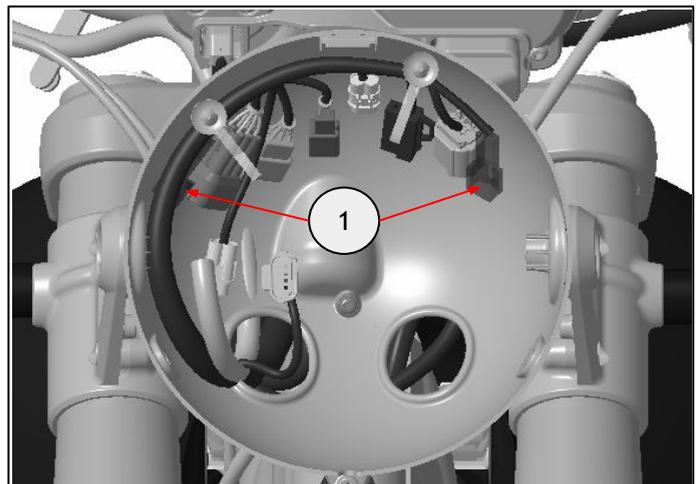
**5** Remove the right hand side headlamp mount (1) by removing the headlamp fixing (2) and the mount fixings (3). Retain for reuse.
