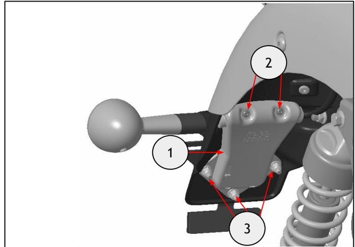
**15** Disconnect the indicator connectors (1). Remove the indicators by removing the nuts (2).
