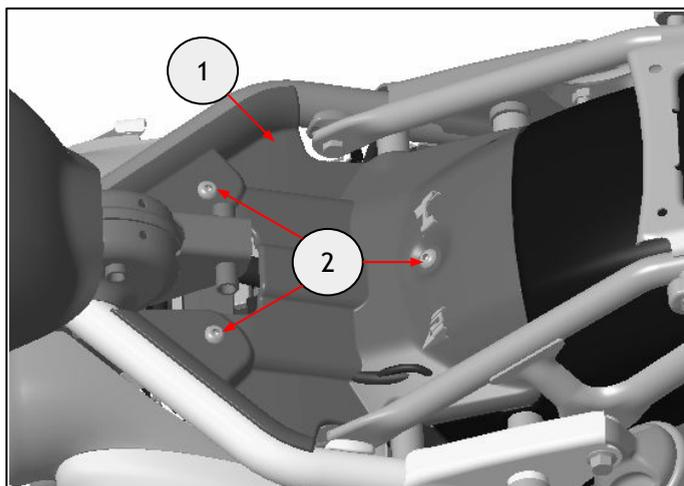
**36** Remove the flasher bracket (1) by removing the fixings (2). Retain for reuse.
