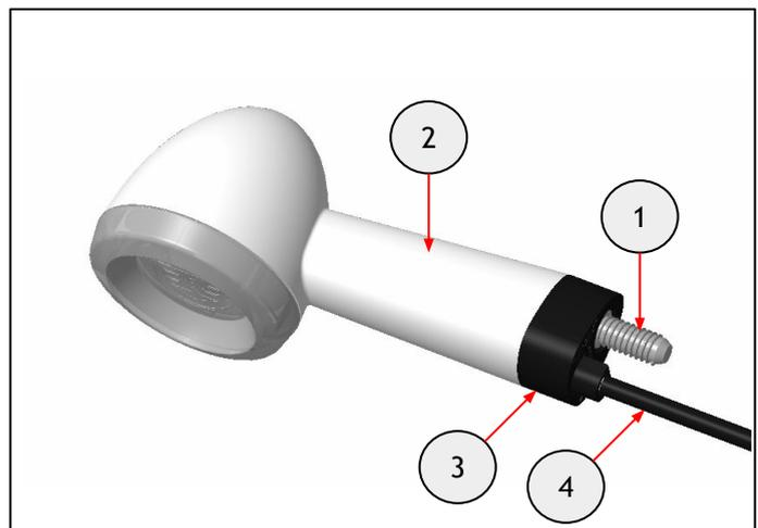
**17** Fit the new indicators on the motorcycle using the nuts (1) removed in step 15. Plug the red connectors together and the green connectors together. While maintaining the indicators in position using a 24mm spanner (2), tighten the nuts to **5Nm**.
