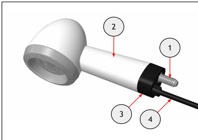
**30** Fit the indicator (1) on the headlamp housing (2) using the nut (3) removed in step 28.
