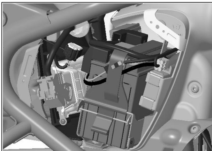
**25** Remove the casquette and headlamp assembly (1) by removing the fixings (2). Disconnect the headlamp connector. Retain for reuse.
