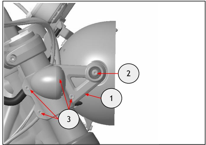
**6** Remove the indicator assembly (1) by removing the fixing (2). Retain both for reuse if the motorcycle is to be returned to its original condition.
