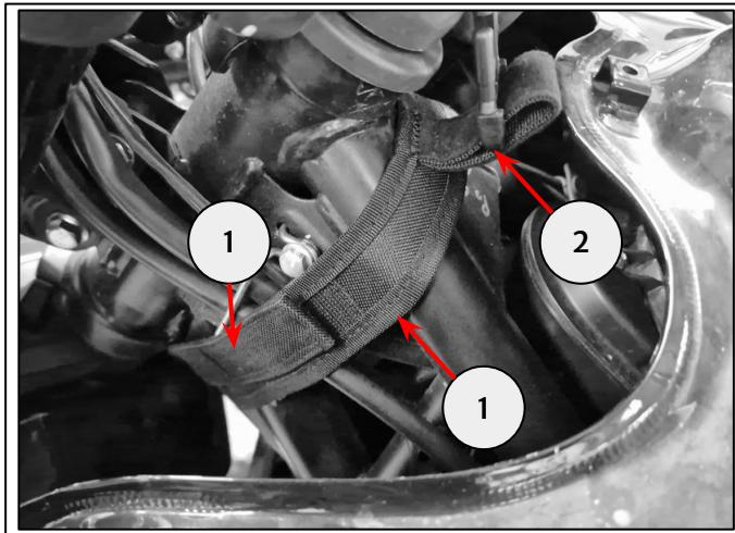
**2** Carefully locate the tank bag onto the fuel tank in order to provide guidance on the location of the magnets. Remove the tank bag.
