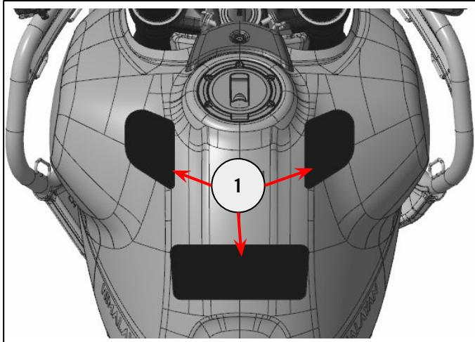
**4** Attach tank bag to the fuel and engage the front safety buckle (1). Conduct a full left to right handlebar sweep to ensure sufficient clearance to the tank bag.
