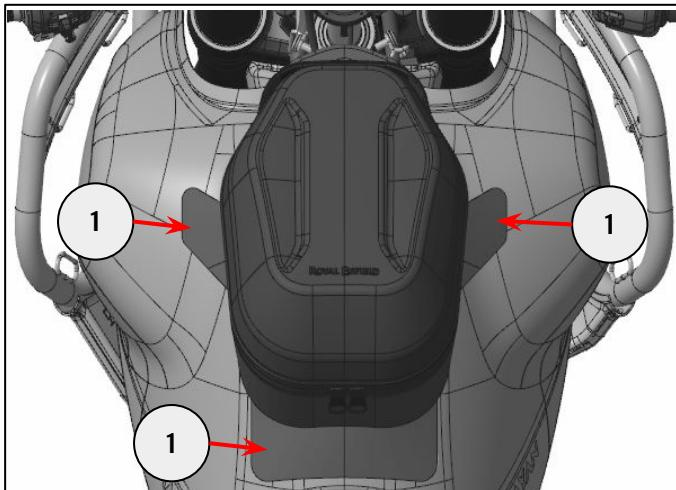
**3** Peel the backing paper and apply the paint protection film to the magnet contact areas (1).
