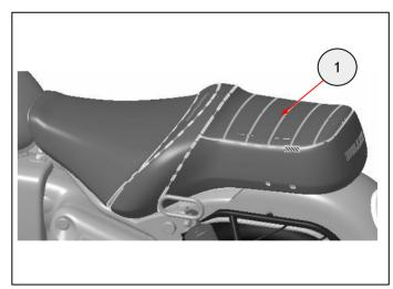
**4** Refit the grab rail (1) and fixings (2) on both the sides. Tighten the fixings (2) to **25Nm** on both sides
