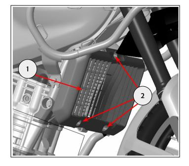
**2** Using the M6 x 14mm fixing from the kit (1), attach the top of the new radiator guard (2) to the top of the radiator (3). Do not fully tighten at this stage.
