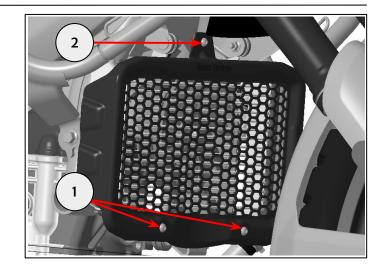
CAUTION: Regularly check the radiator guard for obstruction by insects, leaves or mud. Clean off any obstructions with a stream of low pressure water.
