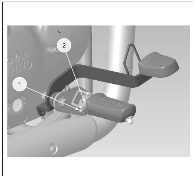
**2** Remove the clevis pin (2) from the footrest clevis and retain for re-use.
