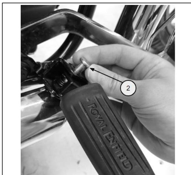
**3** Remove the footrest (3) from the clevis and retrieve the return spring (4).
