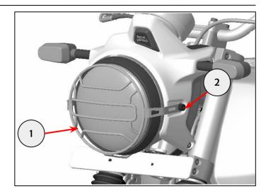
**5** Tighten the lower mount fixing to 5Nm first before tightening the side mount fixings to 18Nm.
