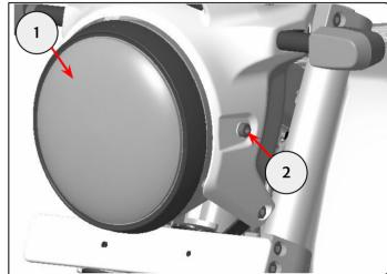
**3** Affix the foam pad on the headlight grill lower mount approximately 45mm distance from shown edge as shown.
