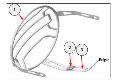
**4** Position the headlight grill to the cockpit area as shown. Assemble an M8 x 40mm fixing from the kit through the side mounts, and an M5 x 12mm (3) through the lower mount. Align and engage all fixings before fully tighten.
